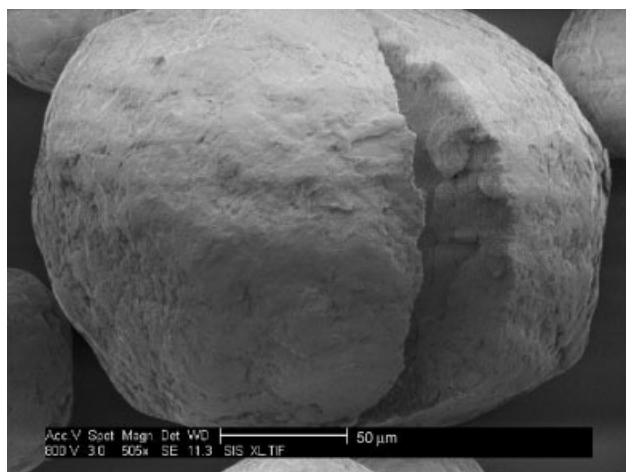
Figure 12 LVSEM observation: fractured nascent POM particle crushed at room temperature.
